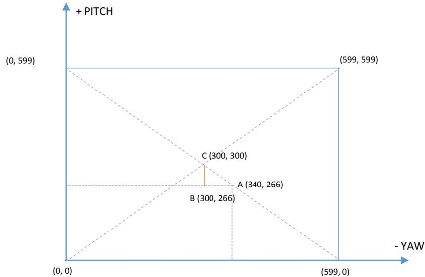
In the current attitude of ASTROSAT, the source is seen by the pixel A(340, 266).
