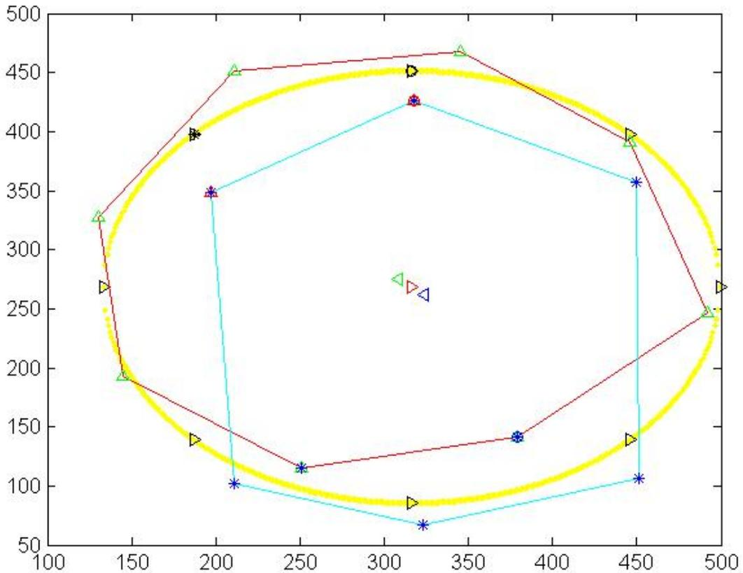
The center computed by taking average errors of both FUV and NUV is (316,268). With reference to this center, a pitch error of +60 pixels and yaw error of +12 pixels is observed. **Thus, for moving this center towards ideal center (256,256), a negative pitch rotation of 60 pixels and a negative yaw rotation of 12 pixels is required.** It is observed pictorially that, the corrected center appears to be in between the centers of FUV and NUV circles.
