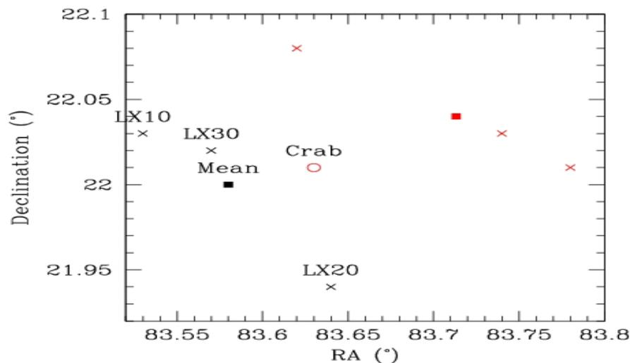
Black points represent the detector position after misalignment correction of September 2015. Red points represent the detector position after misalignment correction in November 2015.
