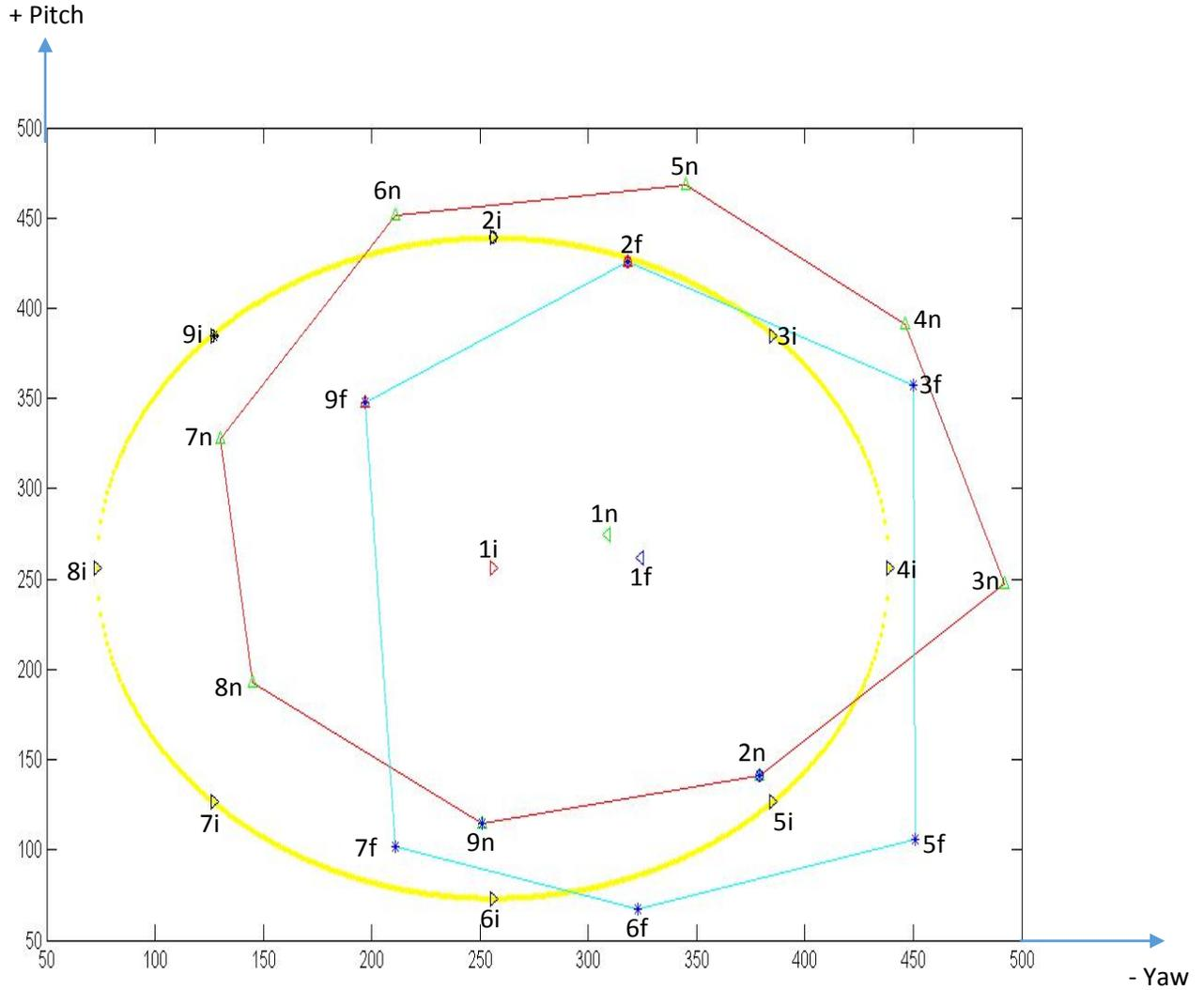
The diagram indicates the 9-point calibration profile circle before the misalignment correction. The radius of the circle is 10 arc min. The circle with red line indicates the actual achieved points for NUV, the circle with blue line indicates the actual points achieved for FUV and the circle with yellow line indicates the ideal points.
