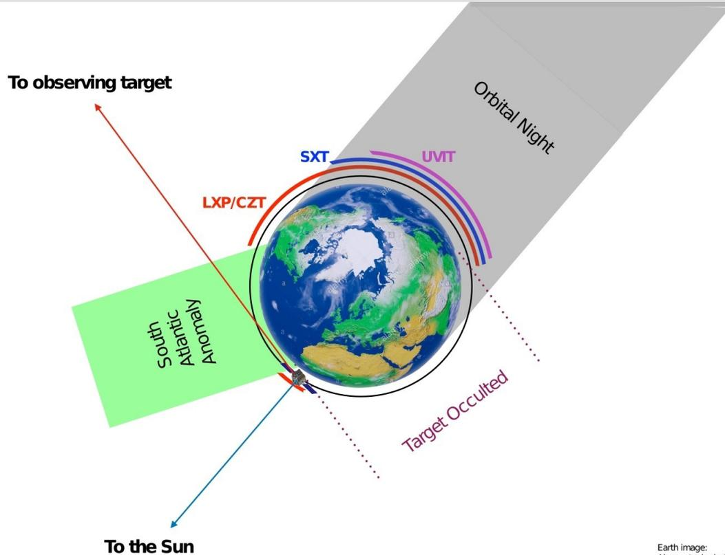
SXT and UVIT can observe only during orbital night. For UVIT there is an additional overhead of switching on after the orbital night begins and switching off before orbital night ends. SXT does not undergo such an on-off sequence.
