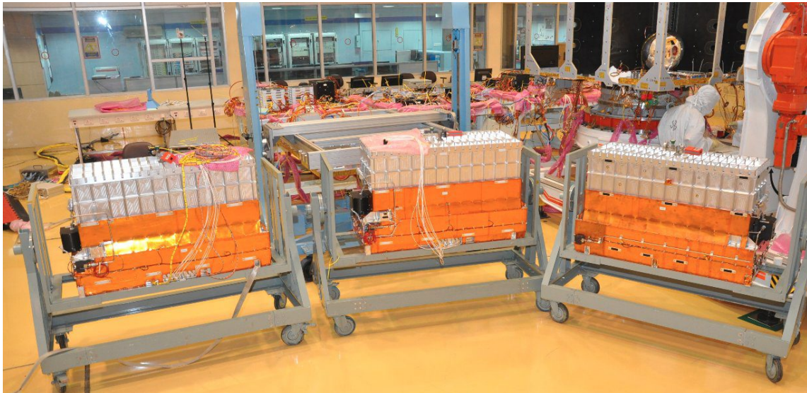
Figure 3: All the three LAXPC Space flight detectors in Assembly, integration and testing lab (AIT) lab after successfully completing all flight tests and final calibration (20 th October, 2014). The purification pump is seen as black box in each detector.
